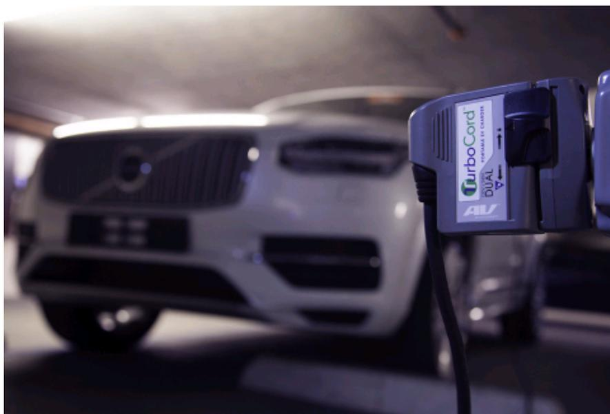
The AeroVironment TurboCord DUAL Charging a 2016 Volvo XC90 T8 at 240volts
