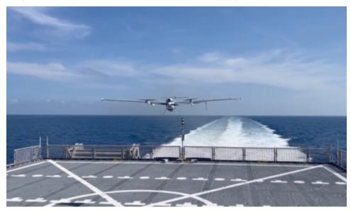
AeroVironment's JUMP 20 VTOL demonstrated autonomous shipboard takeoff and landing during the U.S. Navy's Hybrid Fleet Campaign Event in Key West, FL (Photo: AeroVironment, Inc.)
